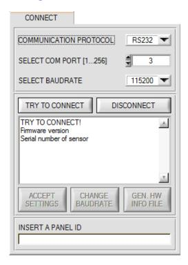
When a connection is established the serial number of the contacted sensor is transferred in addition to the firmware version
