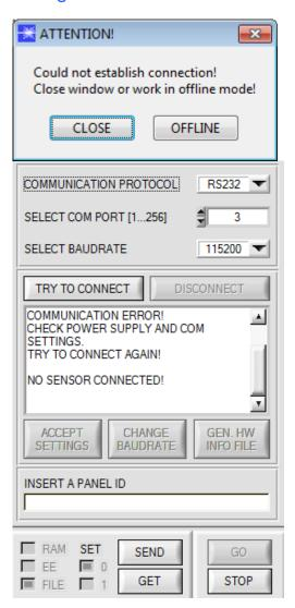
If a connection is not established automatically, e.g. if no sensor is connected, the software can be run in OFFLINE mode. In offline mode it only is possible to exchange parameters with a file on a storage medium, which often is helpful for the purpose of analysing parameter files.
