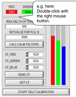
Accessing offset calibration now requires a double-click with the right mouse button exactly on the frame in the CALIB tab.
